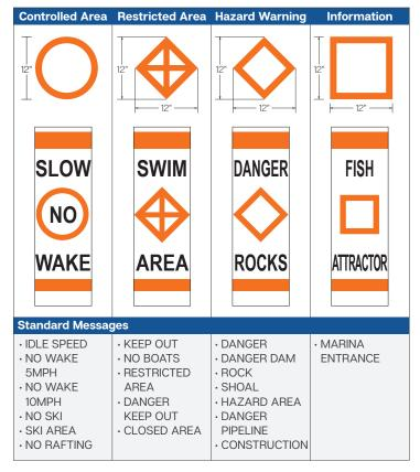
For SL-B700-RB, SL-B1060-RB, SL-B1200, SL-B1250, SL-B1362-RB, SL-B1428EB, SL-B1452, SL-B2445 where 12 inch orange symbol is standard. SL-B576 graphics will be vertical due to minimal width and require 5 inch orange symbol.
