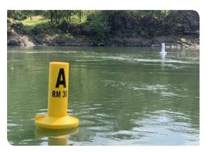
Fast moving rivers of the Pacific Northwest are one deployment site for a state marine agency. The SL-B700 features a slight fin on it's keel which helps keep the buoy in the water current thus reducing drag on mooring chain and cable.
