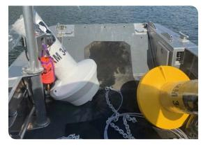
A lifting eye located on top of the float collar makes deployment and retrieval easier and safer. The lifting eye connects to the mooring eye on the bottom of the buoy via 316 stainless rod for enhanced strength and stability.
