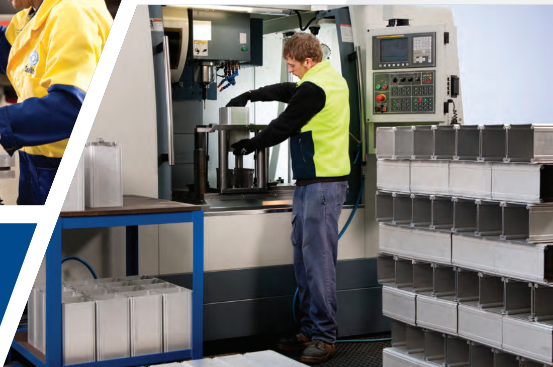
Sealite solar chassis processed through CNC
