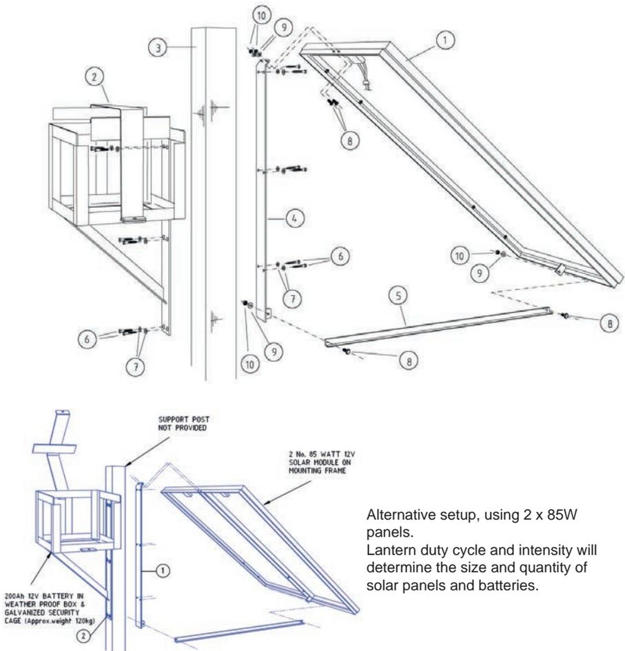
Alternative setup, using 2 x 85W panels.
