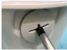
2. Gently insert the SIM into the holder. Make sure the SIM Card is positioned correctly.
